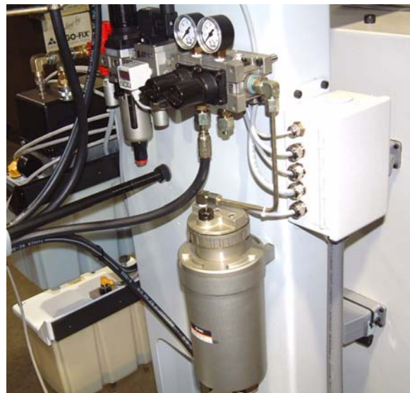
Filter Regulator Package (Located on Barfeeder)
