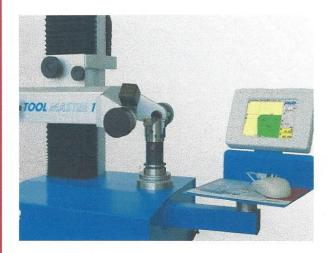
TM10-TCAM2 is the entry model for tool measuring with electronic image processing It is the intelligent combination of a digital CMOS-camera and evaluation electronics with a 6.4" TFT-colour monitor.
